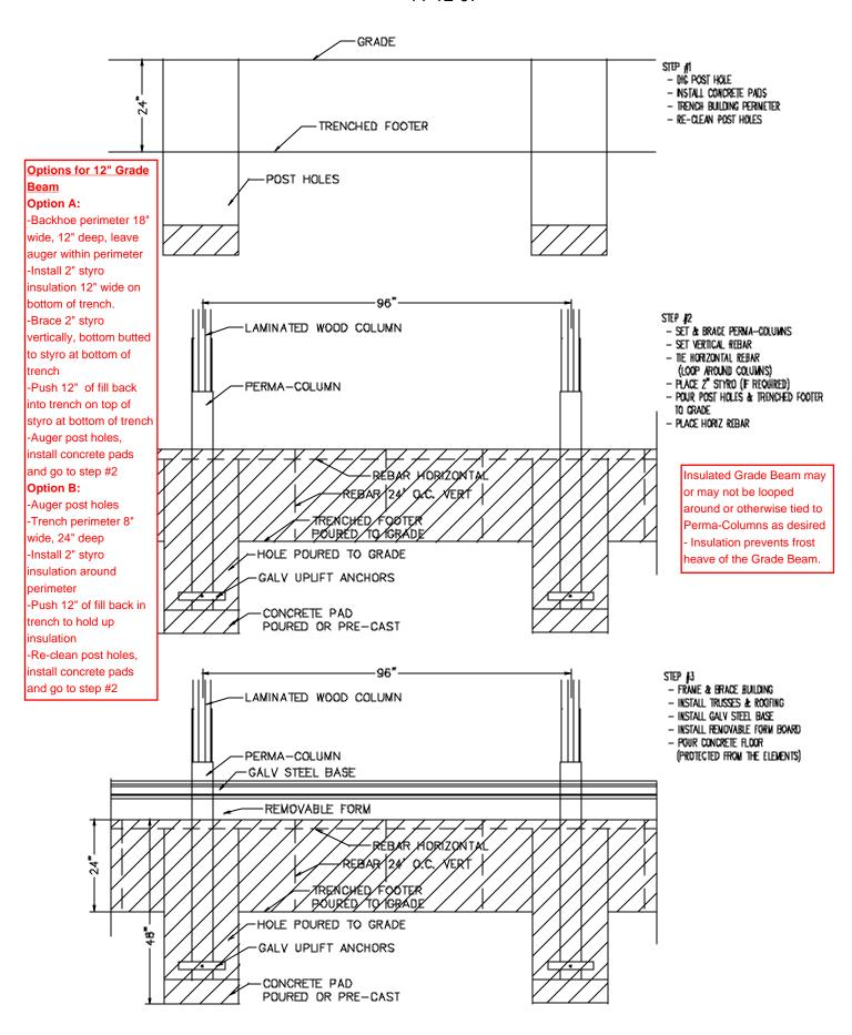
Photo illustration of the least expensive of all continuous concrete foundation options using Perma-Columns:
